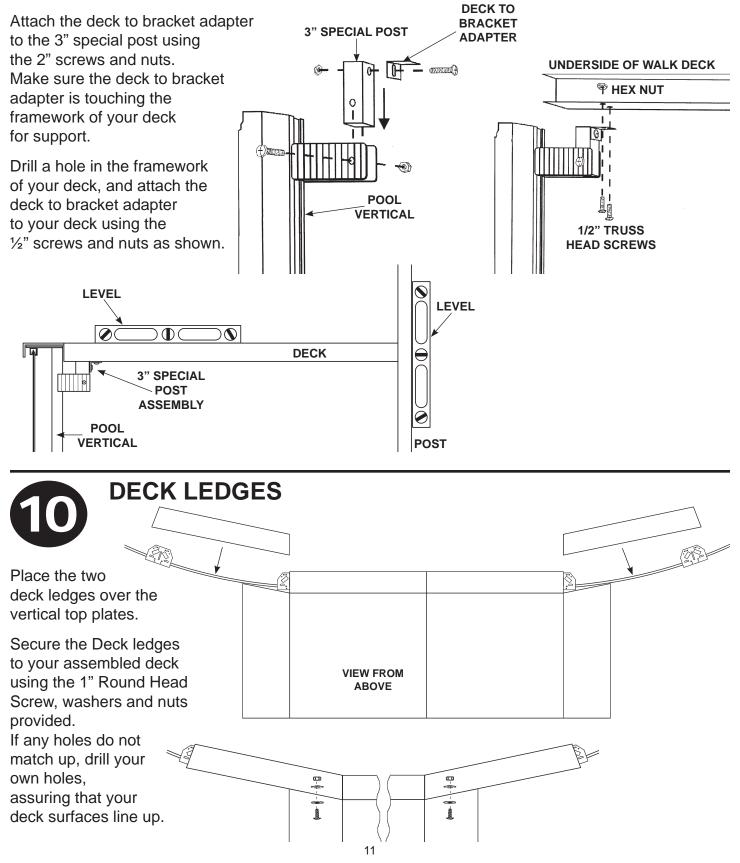
Secure the two deck ledges and the ledge section of each 4'x5' patio to the top plates.
